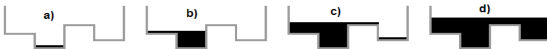
Picture 2: a) Valley basin, b) Lake filling, c) Overflowing and d) Neighbor connecting.
